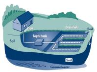
water long enough to allow all solids to settle out (forming sludge) and oil and grease float to the surface (as scum). Compartments and a T-shaped outlet in the septic tank prevent sludge and scum from leaving the tank. Screens are also recommended to keep solids from entering the drainfield.
