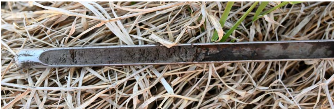
Figure 32. View of a hand core showing soil profile within the red canary grass restoration area.
