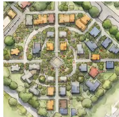
COTTAGE COURT - Example of a Cottage Court style development where a cluster of small scale cottages are arranged around shared open space and parking areas on a relatively small plot of land.
